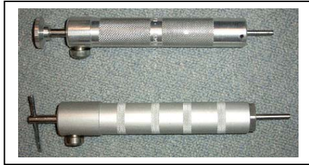
Figure 5: Spring operated captive bolt guns for stunning rabbits (Photo: I. Schuett-Abraham)
