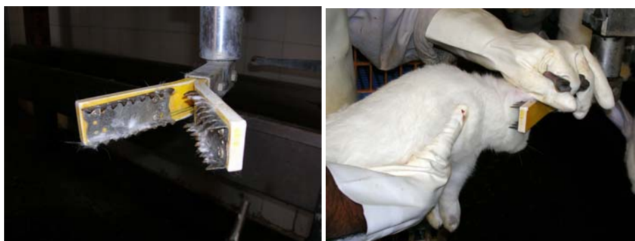
Figure 6 a + b: Electrical device for stunning rabbits (Photos: S. Diverio)
