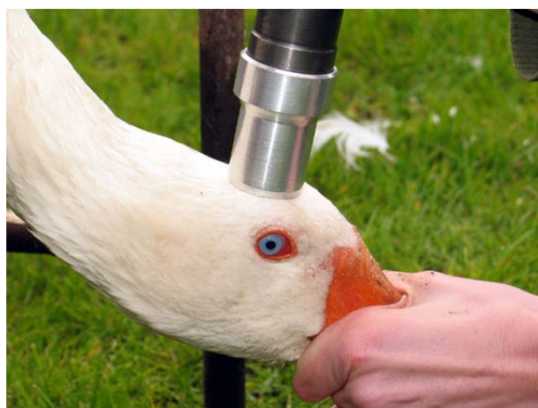
Figure 11: the correct positioning of the “Cash” Poultry Killer for geese.
