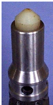
Figure 9: Convex head of percussion stunner for ducks (Photo: Leisha Hewitt)
