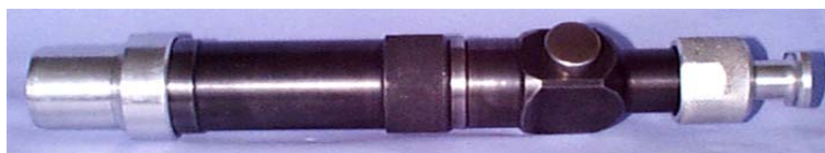
Figure 8: Percussion stunner for poultry (Photo: Leisha Hewitt)
