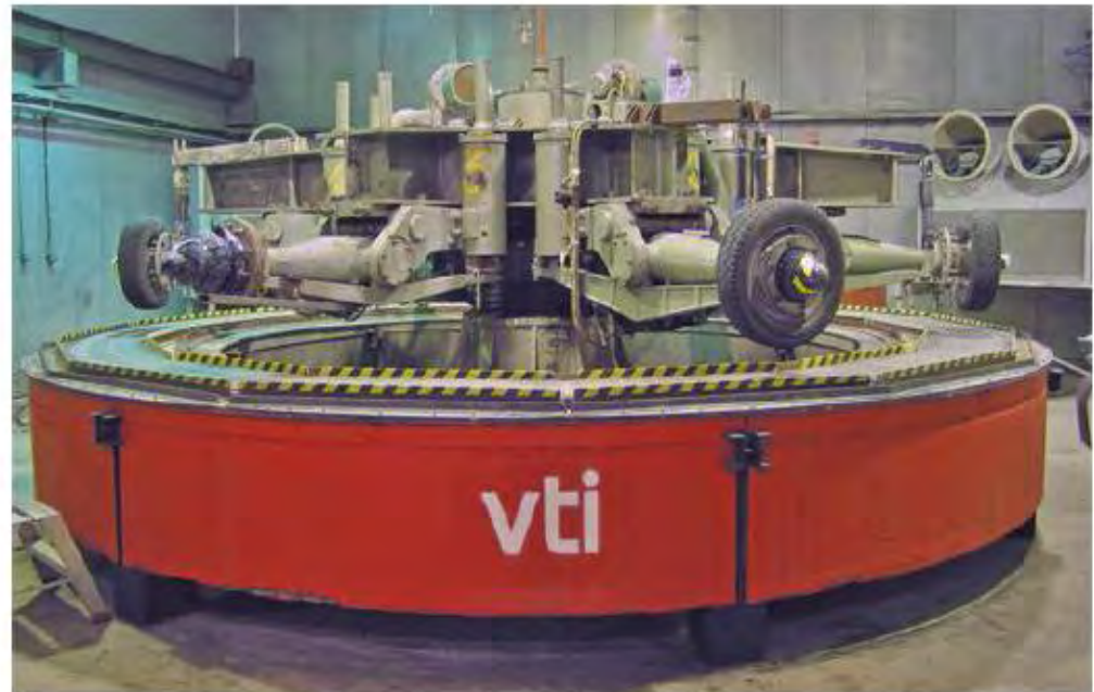
Figure 7. VTI road test machine for abrasion and particle studies
